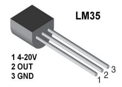
The LM35 series are precision integrated-circuit temperature devices with an output voltage linearly-Factor proportional to the Centigrade temperature. The LM35 device has an advantage over linear  $-55^{\circ}$ C to 150°C Range temperature sensors calibrated in Kelvin, as the user is not required to subtract a large constant voltage from the output to obtain convenient Centigrade scaling. The LM35 device does not require any external calibration or trimming to provide typical accuracies of
