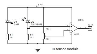
IR sensor consists of an IR transmitter LED and a photodiode at the receiver end. The photodiode converts the light into current which is converted into voltage and which is compared against a fix voltage to get the output. The main problem with the IR sensor is its range. The range of IR sensor can easily be increased by the adjusting potentiometer at the receiver end.
