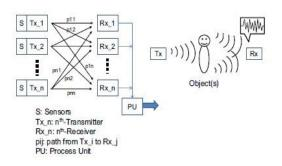
As shown in figure and according to [7] RSSI system requires large number of RF signal transmitter and receiver. The basic disadvantage of RSSI system is its
