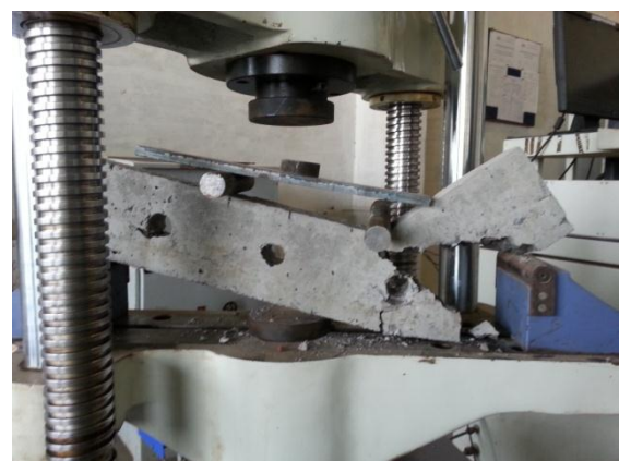
Fig. 5 Casting and testing of beam with three opening.
