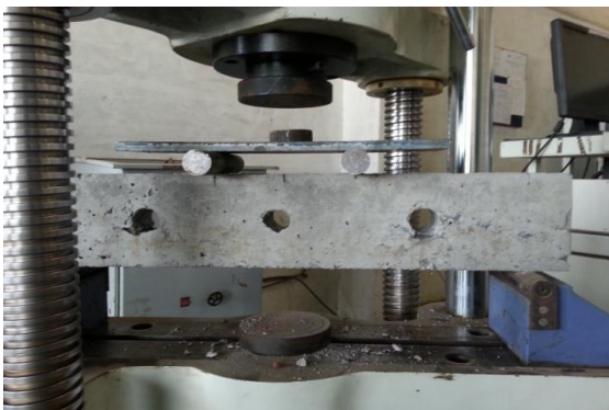
Fig.6 Typical arrangement of two point loading condition.
