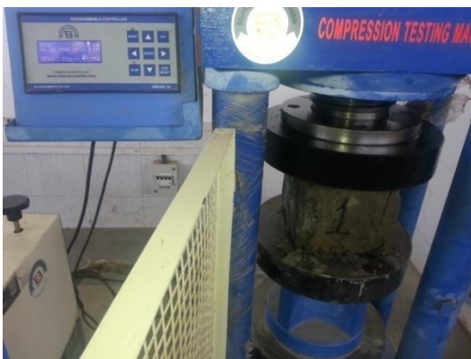
Fig. 3 Testing of Cubes.
