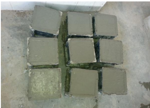
Fig.2 Casting of cubes.
