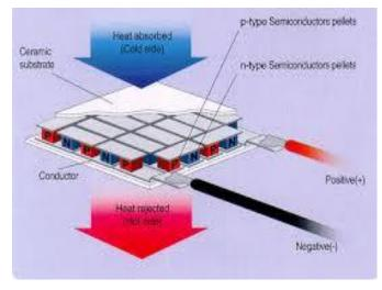
Fig -1: Thermoelectric Module
