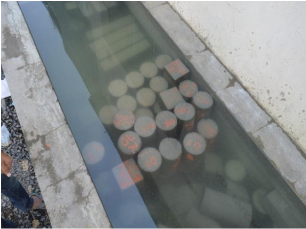
Fig -2 Specimens are kept for Curing in Curing Pond
