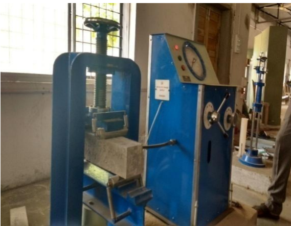
Fig -3 Testing of prism in flexural Testing Machine
