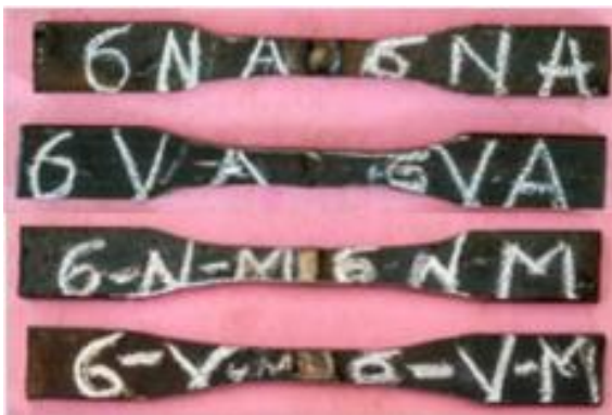
Fig -3.5:6mm Thick Plate Tensile Test Specimens
