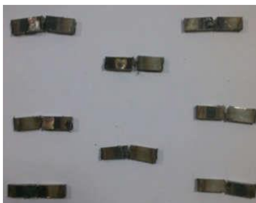
Fig -3.7: Specimens after Charpy Impact Testing
