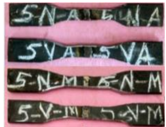
Fig -3.4: 5mm Thick Plate Tensile Test Specimens
