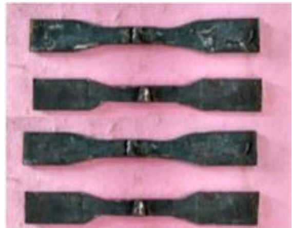
Fig -3.3: 4mm Thick Plate Tensile Test Specimens
