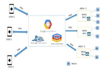
Fig -1: System Architecture
