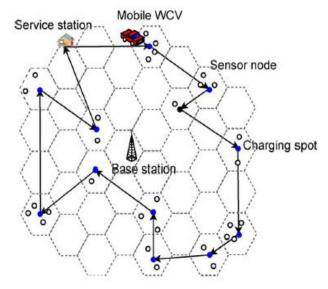
Fig 1: Sensor network with mobile WCV
