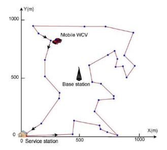
Fig 3. Optimal travelling path for the sensor network
