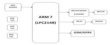
Fig3: Block Diagram
