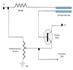
FIGURE NO.3 Sensor design\_Equivalent diagram of soil moisture sensor
