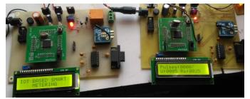
**Fig-4:** Output of Meter 1 is being sensed and transmitted. Data is locally displayed on the LCD panel
