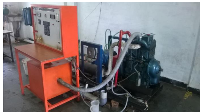
Fig -2: Twin cylinder 4 stroke diesel engine test rig with hydraulic dynamometer loading.
