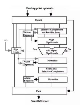
Fig 3. Block diagram of Adder/Subtractor
