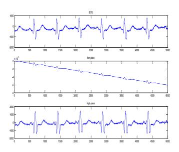
**Fig -3:** Results of Tompkins filter (a) nosy ECG (b) after Low pass filter (c) output of High pass filter
