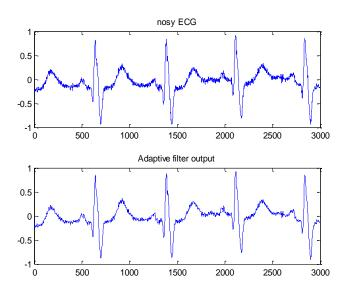
**Fig- 7:** Adaptive filter (a) nosy ECG signal (b) output of adaptive filter
