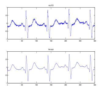
Fig- 8: results of LMS + low pass filter
