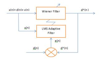
Fig- 6: Adaptive LMS filter block diagram
