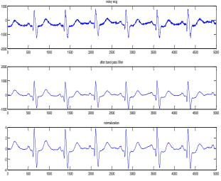
Fig- 4: Results of Butterworth filter (a) nosy ECG signal (b) Output of Butterworth
