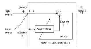
Fig- 5: Block diagram of Adaptive filter
