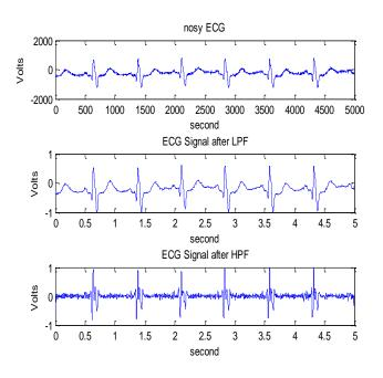
Fig- 2: Output of Savitzky-Golay filter (a) nosy ECG signal (b) output of LPF (c) HPF
