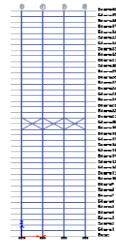
Fig -5 :Elevation showing X-shape belt truss
