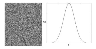
Fig-1: (a) Gaussian noise image (b) Gaussian noise distribution
