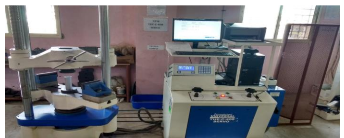
Fig -2: Quasi static test set up using Fine Spavy UTM
