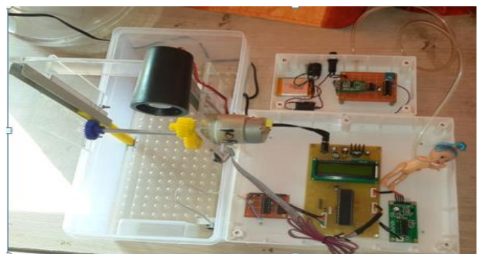
Fig -4.3: Prototype of automated drowning detection system with swimming tub
