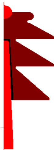
Fig-1: axis symmetry view of 11KV insulator
