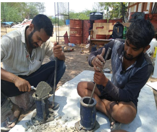
Figure - 3.0 Casting of GPC Cylinders.
