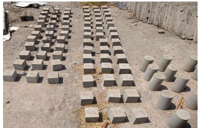
Figure - 4.0 Specimens curing in Ambient Temperature.
