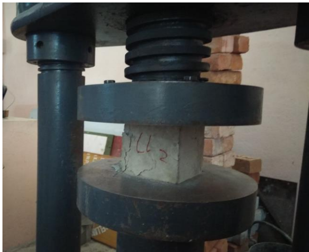
Figure - 5.0 Compressive test on concrete cube.
