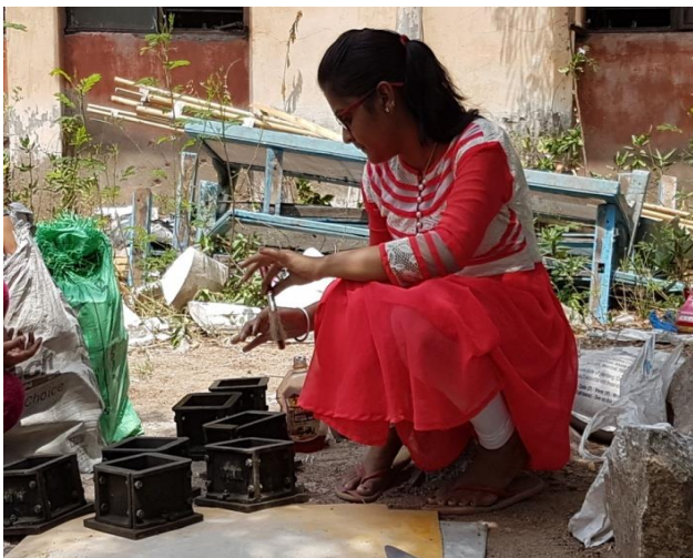
Figure - 2.0 Cube specimens prepared for casting.
