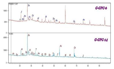
XRD analysis of the G-GPC's Specimen showed the presence of Quartz, Analcime, Anorthite, Mullite, Jadeite and Albite. The G-GPC specimens exhibits peaks of syngenite. Peaks of Thenardite are also observed. Thenardite occured due to reaction between Na ions form the NaOH solution with sulfate ions leading to the formation of sodium sulfate decahydrate.
