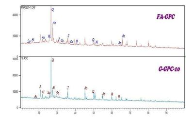
In the x-ray diffraction analysis of trail-1 specimens, GGBS
