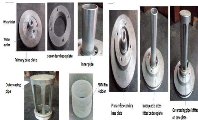
Fig-1: Micro channel heat exchangers Parts & Assembly
