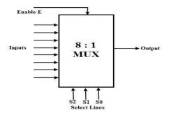
Figure 3.4: Block diagram of 8:1 MUX
