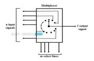
Figure 3.3: General working of MUX
