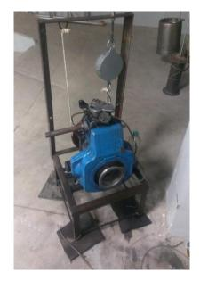
Fig.12 Engine with Rope brake Dynamometer
