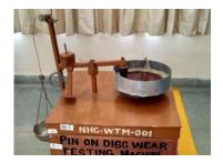
Fig. 5 Pin on Wear testing machine
