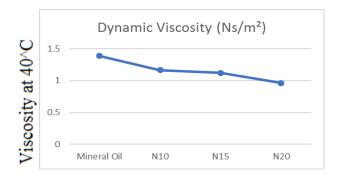
Fig. 10 Dynamic viscosity of different blends of oils ( $x10^{-4}$  Ns/m<sup>2</sup>).
