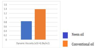
Fig. 8 Dynamic or Absolute viscosity of the oils.
