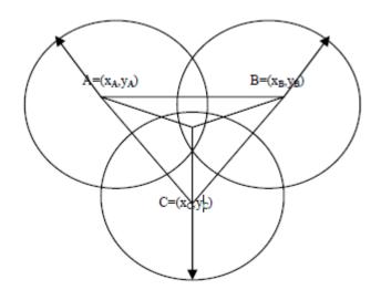
Figure-5: Position Approximation Algorithm
