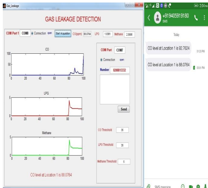
Fig -6: Data Acquisition from Sensors using GUI
