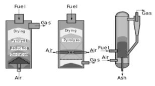
Fig -4: Updraft, Downdraft, Fluidized bed gasifiers
