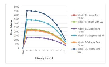
Graph No.3 Base Shear of all models in X-Direction in KN.
