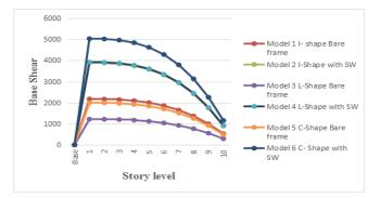
Graph No.4 Base Shear of all models in Y-Direction in KN.
