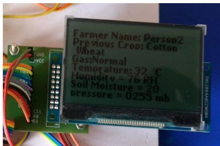
Fig -7: Display of person2 farm information on GLCD
