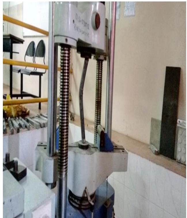
Fig. 5. Failure modes of circular column
