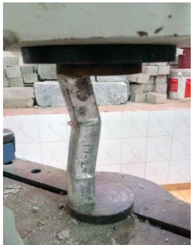
Fig. 6. Failure modes of square column
