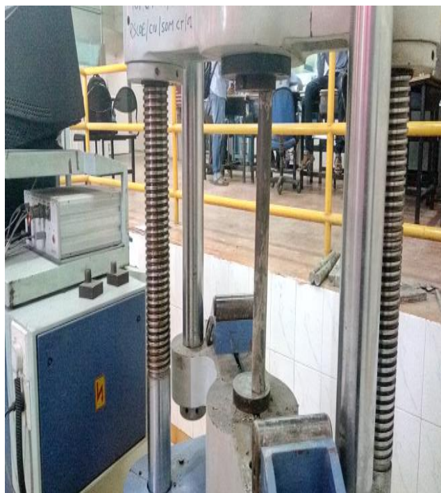
Fig. 4. Arrangements of CFST circular column in UTM
