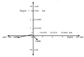
The amount of  $x_1$ ,  $x_2$ ,  $x_3$ ,  $y_1$ ,  $y_2$ ,  $y_3$  (in degree) can be converted to km and inserted in (1) through (3), then x4 and y4 are obtained in kilometer unit, then, they are converted to a degree from the process which were discussed in the current section and, finally, the user can identify its own position.
