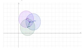
Fig -2: Coverage area of triple DME
