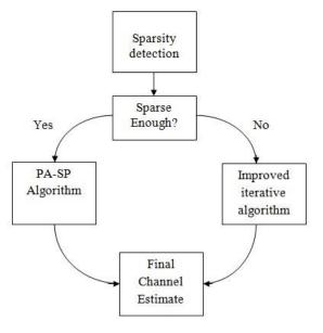
Fig-3. Structure for adaptive channel estimation
