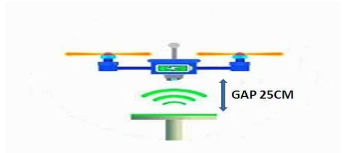
Fig -5: UAV charging through WPT
