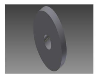
Fig 4 :- Inventor Model of SHM Cam
