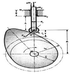
Fig 3 :- Force Acting On Cam And Follower Given Data:-
