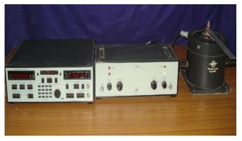
Fig 1:- Vibration Exciter With F.F.T
