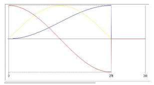
Blue – displacement , Yellow – velocity , Red- acceleration Graph 2 :- Graphs For Snail Cam
