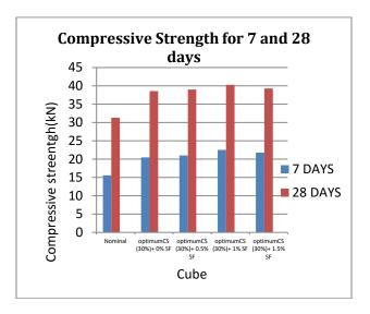
Fig.8: Compressive strength for 7 & 28 days
