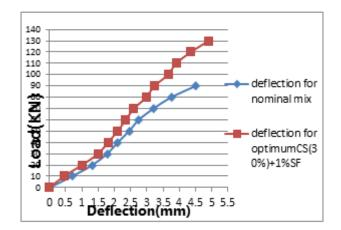
Fig 14: Load vs deflection cure for beam
