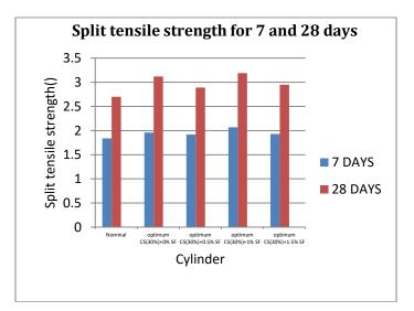
Fig.9: Split tensile strength for 7 & 28 days
