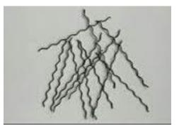
Fig.2: Crimped steel fibers
