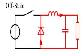
Fig -4: Buck Converter OFF State
