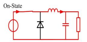
Fig -3: Buck Converter ON State
