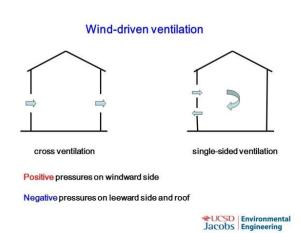
Fig. Wind Driven Ventilation
