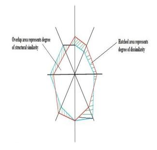
Fig. 2.(c) Super imposed Polar plot of the row sum of [WSSP] matrix for kinematic chain 1(a) and 1(b) as shown in Fig. 1
