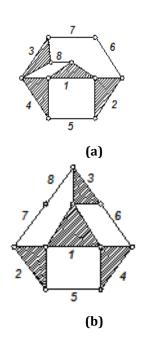
Fig. 1 (a) and (b) 8-links, 10-joints, 1-F kinematic chains
