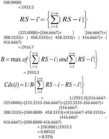
Coefficient of structural similarity between two kinematic chains shown in fig is determined using equation as
