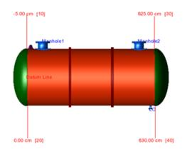
Fig:-1 Mounded pressure vessel with stiffening rings
