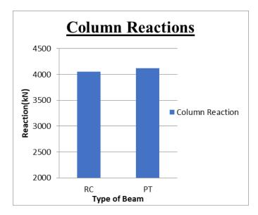
Fig.4.3 Base Reactions of column
