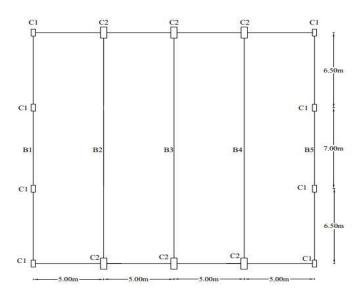
Fig.3.1 Geometrical plan of floor system
