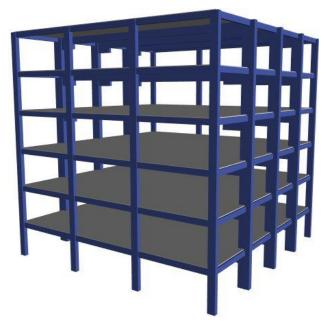
Fig.3.2 Six Storeyed RC Frame System
