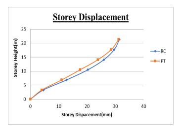
Fig.4.4 Storey Displacement
