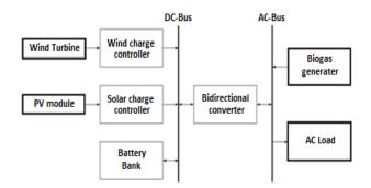
Figure-1: Circuit Diagram of Solar-Wind-Biogas Hybrid System
