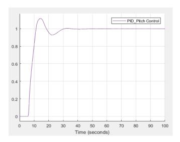
Figure 7:The unit step response of wind turbine with PID controller
