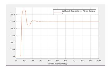
Figure 6:The unit step response of wind turbine without controllers
