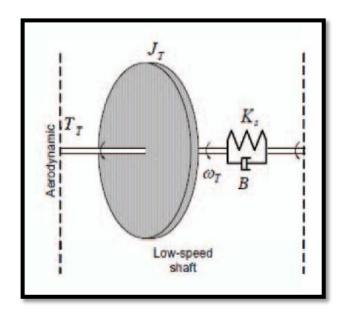
Figure 2: Mechanical model of drive train
