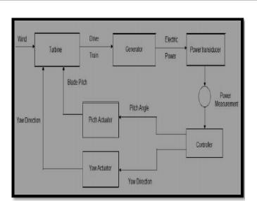
Figure 1: Wind Turbine System Feedback Control System Model
