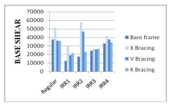
Fig.14. Comparison of base shear
