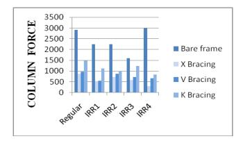
Fig.16. Comparison of column force
