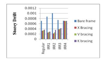
Fig.12. Comparison of storey drift in x direction
