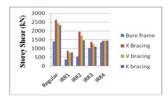
Fig.8. Comparison of storey shear in x direction
