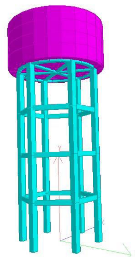
Fig - 4: 3-D Elevated Circular tank
