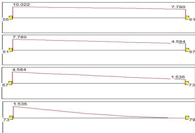
Graph- 3: Showing Deflection curves and Displacement values(in mm) for Circular tank for ZONE II
