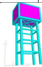
Fig - 3: 3-D elevated Rectangular water tank
