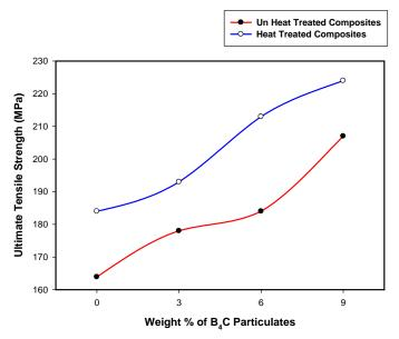
Figure 3: Ultimate tensile strength of AA7030-B<sub>4</sub>C composites with and without heat treatment
