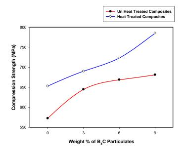
Figure 5: Compression strength of AA7030-B<sub>4</sub>C composites with and without heat treatment
