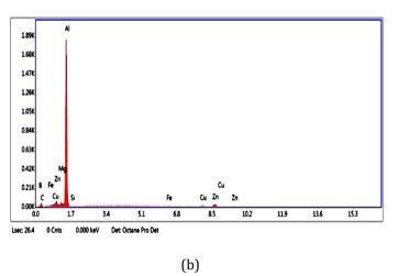
Figure 2: Shows the EDS graphs of (a) as cast AA7030 alloy (b) AA7030-9% B<sub>4</sub>C composites
