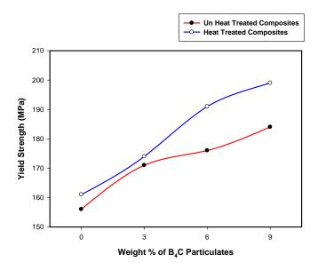
Figure 4: Yield strength of AA7030-B<sub>4</sub>C composites with and without heat treatment
