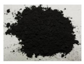
Fig -1: Copper oxide (CuO) in form of nano powder
