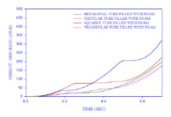
**Chart-2** Energy absorption plot for metallic tubular structure filled with foam
