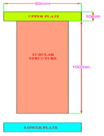
Fig-1 Geometric model of tubular structure
