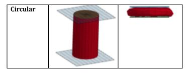
Fig-5 Tube structures before and after loading for metallic tubes filled with foam
