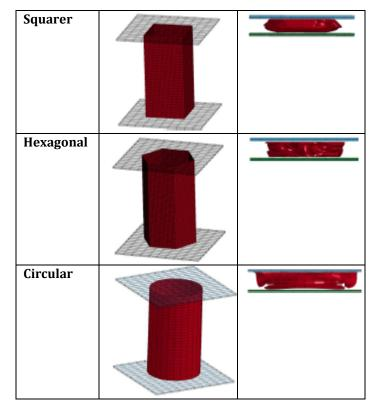
Fig-4 Tube structures before and after loading for metallic tubes
