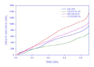
Chart-1 Energy absorption plot for different metallic tubular structures
