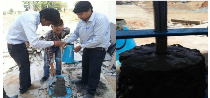
Figure- 1: Measure of slump value in concrete.
