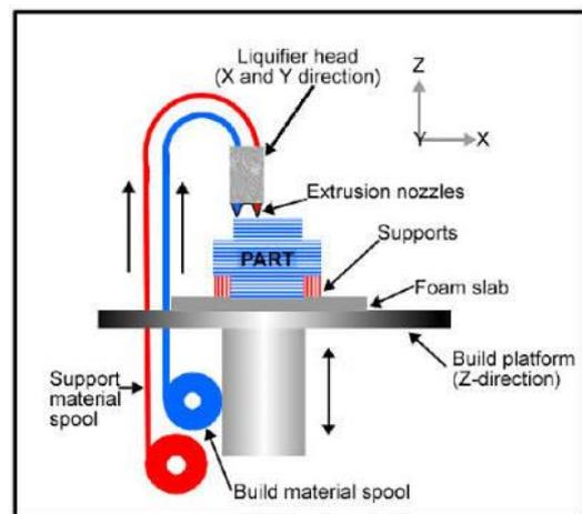
Fig -1: Schematic Representation of FDM Process
