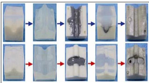
Fig -7: Process flow for improving surface quality of core and cavity of wax injection tool fabricated by FDM [13]
