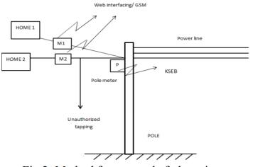
Fig.2: Method for power theft detection
