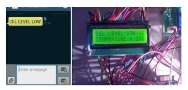
Fig-8: Oil level low detection
